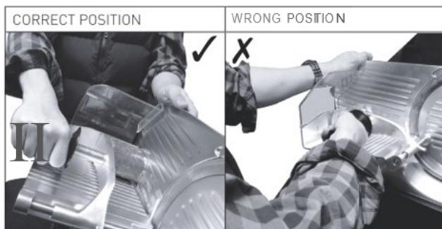
WARNING: no body part should ever come in contact with the rotating blade. For safety reasons, never operate this machine with loose hair or clothing.
