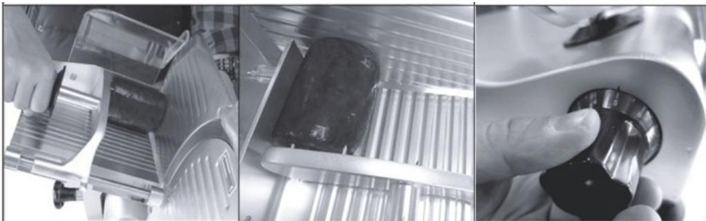
NOTE: operator must face the machine and stand correctly. The right hand shall hold the pusher and the left hand set beside the slide deflector. The user's body must stand perpendicular to the working surface of the slicer.
